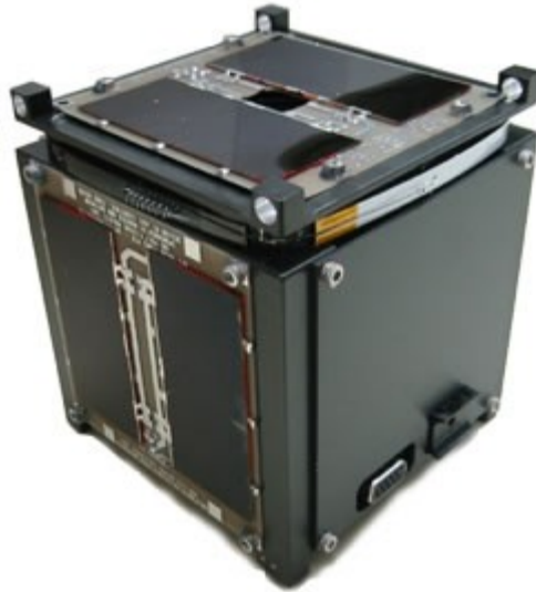
Figure 1 – A completed Cubesat satellite. This model was developed by California Polytechnic State University.
